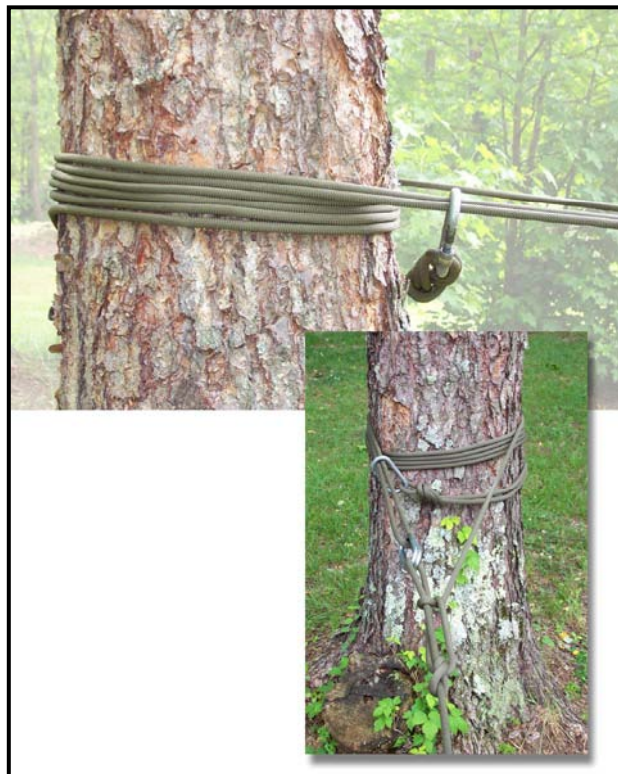
Figure 7-13. Tensionless anchor knot.
